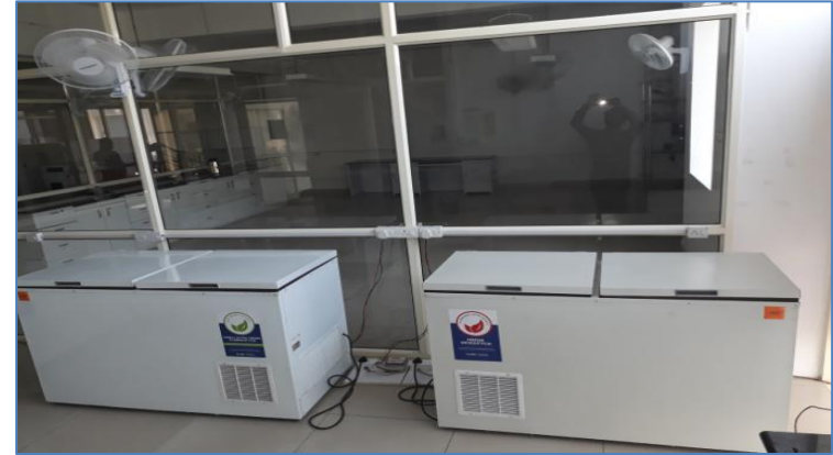
Chest Freezers- with and without PCM, installed at Fare Labs (NABL accredited lab), Gurugram
