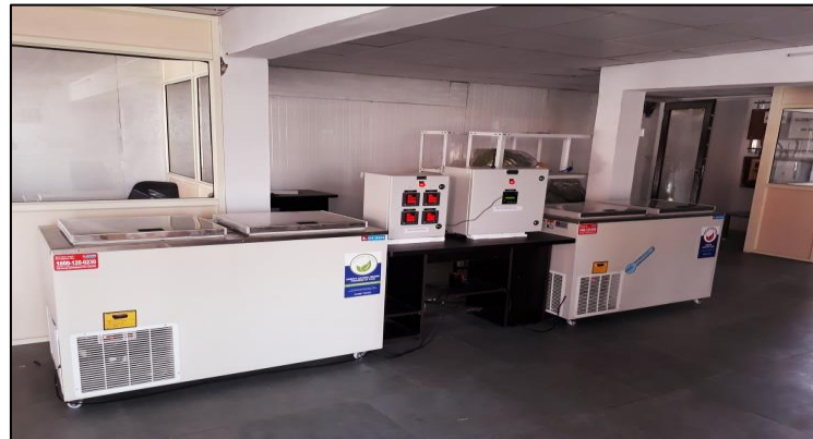
With and without PCM freezers installed at ICEMAKE Refrigeration, Ahmedabad
