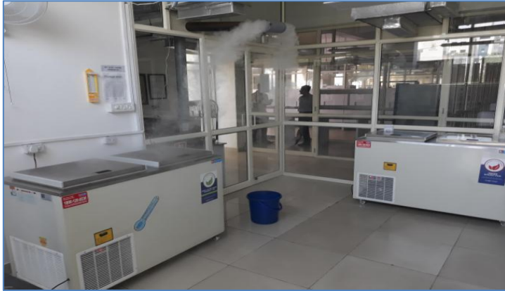
Chest Freezers- with and without PCM, installed at Fare Labs (NABL accredited lab), Gurugram
